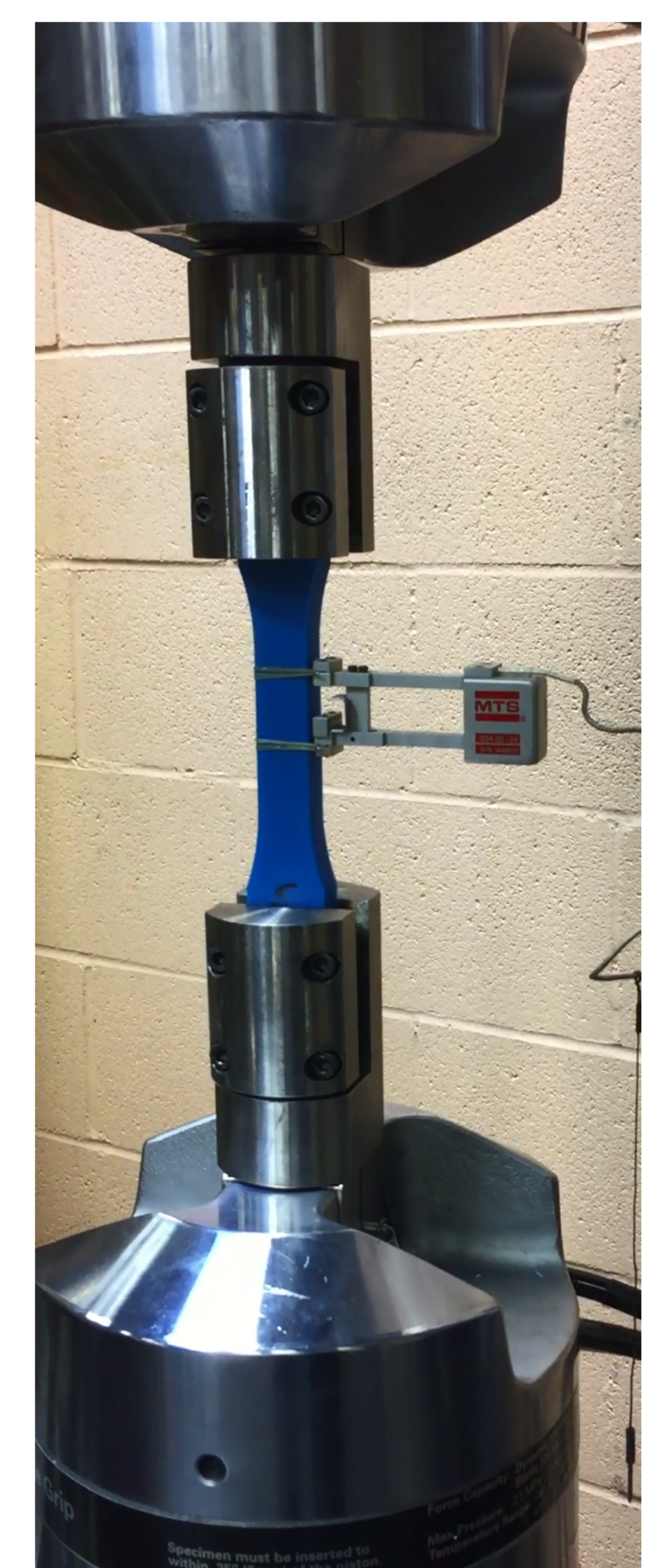
Supplementary tests were also conducted on 3D printed ABS dog-bone samples to determine tensile strength properties
